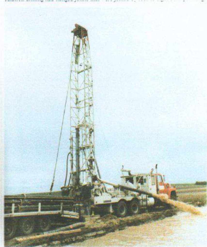
Figure 10.27. The settling pit for a reverse rotary rig is considerably larger than for a direct rotary machine because fluid losses in the borehole are always much higher. The pit should contain at least three times the volume of the material to be removed during drilling. (Portadrill, Inc.)
